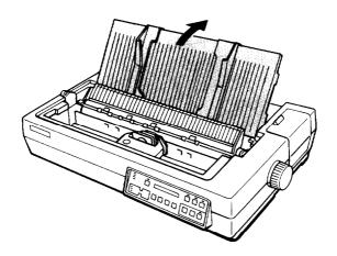
**3.** Align the pins of the paper guide cover with the slots **on** the printer and attach the cover.
